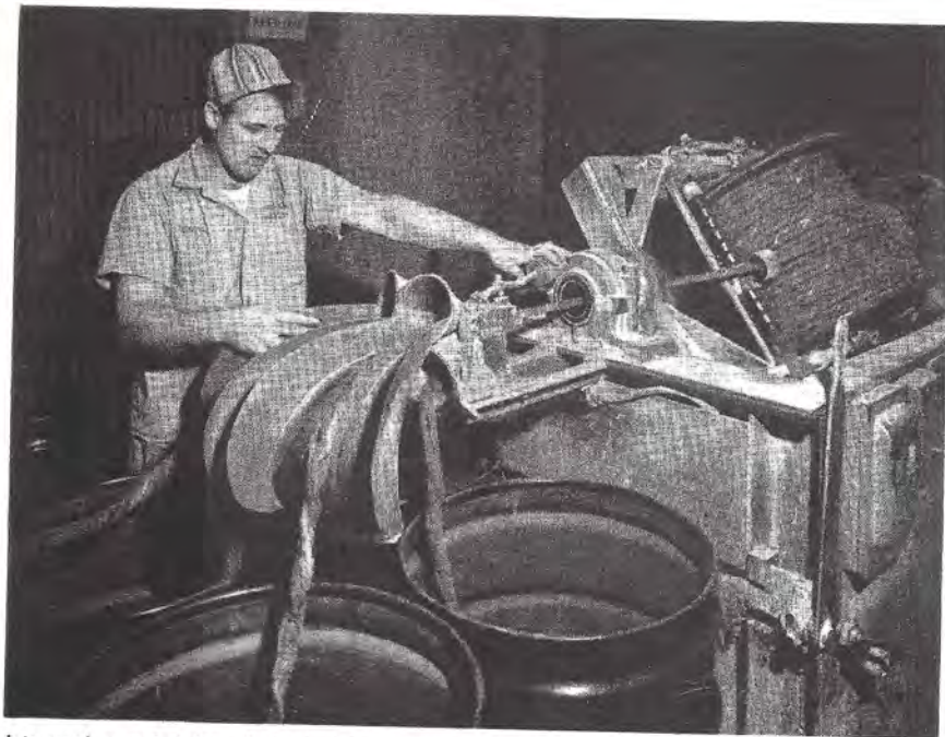
Jute cords are fed from individual barrels to the twisting machine. As the steel spool visible in rear revolves, cords are twisted into four-ply rope. The spool can hold about 100 pounds of rope.
