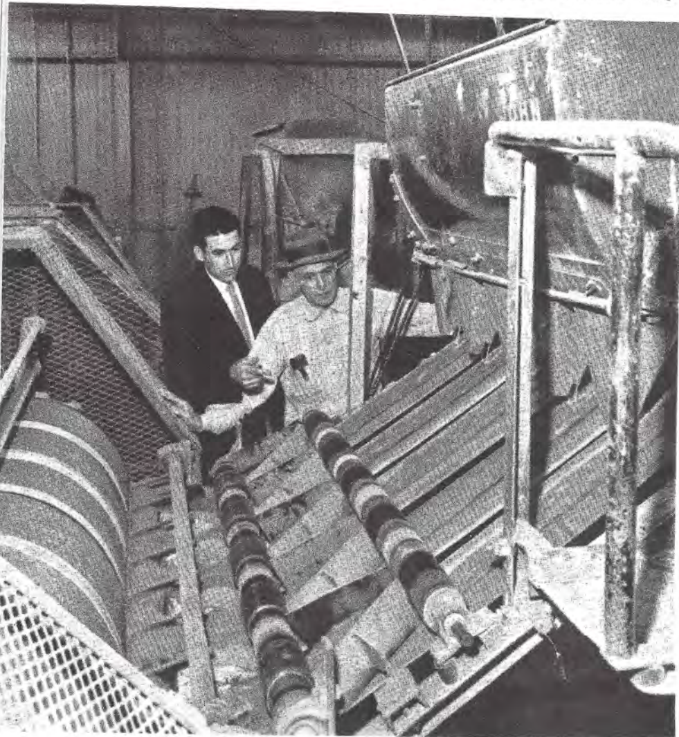
Above, jute is fed onto belt which carries it into picker. Inside, the jute is cleaned of dust, dirt and other debris. Below, jute cords come from a cording machine. Observing are Charles J. Wolford, left, Esso representative, and Jay E. Tollstrup, right, Nupak production manager.
